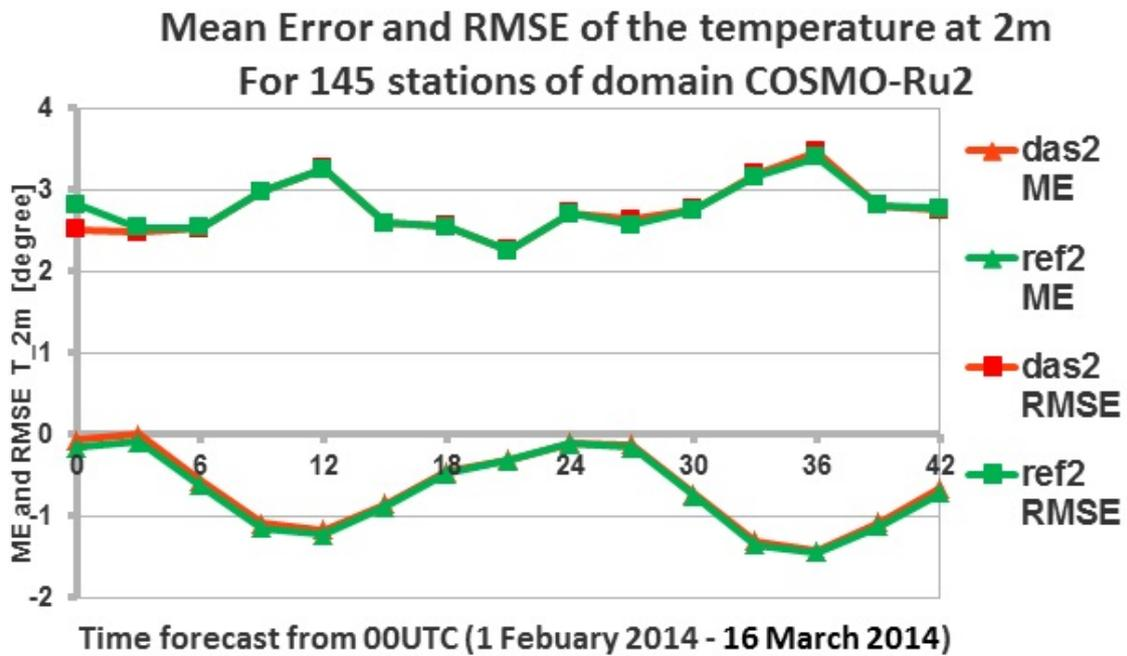
Figure 1: Mean error (ME) and Root Mean Square Errors (RMSE) of forecasts COSMO-Ru2 with DAS (red line) and without (green line) for PMSL,  $T_{2m}$ ,  $Td_{2m}$  and wind speed respectively for Olympic period 1 February – 16 March 2014
