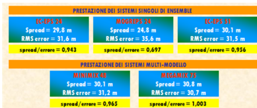
Figure 15: Synthesis of the performance for single-model and multi-model systems in terms of Z500 rmse and spread.
