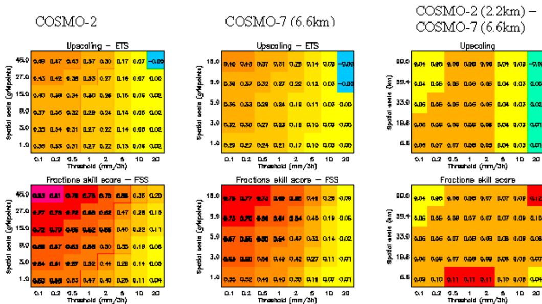
Figure 8: Verification results for the two methods UP (top row) and FB (bottom) and the period from June to November 2007 (3h accumulations). Displayed are the skill scores for the COSMO-2 (left), COSMO-7 (middle) and the differences between those two (right). For the latter, the spatial scale of the COSMO-7 in terms of gridpoints has to be multiplied by 3 to get the comparable spatial scale of COSMO-2.
