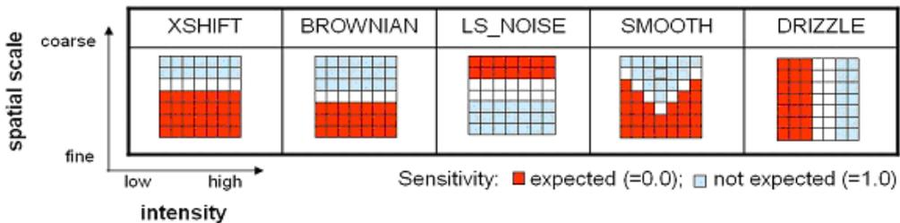
Figure 5: Expected response to the perturbations. Red boxes indicate that a response is expected on these scales why blue boxes indicate scales where no sensitivity to the perturbation is expected. When applying XSHIFT, for example, the verification results are expected to be sensitive for small scales and all thresholds.
