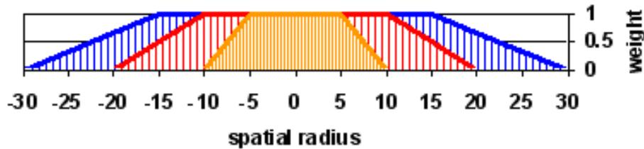
Figure 19: Weights of grid cells depending on the distance from the central cell, for three different sizes of the neighborhood. Blue: Zone of equal weight and fading zone with 15 grid points radius each; red 10; orange: 5.
