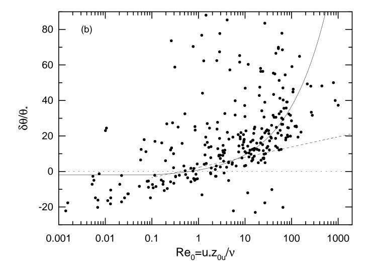
Dimensionless temperature increment across the roughness layer,  $\delta\theta/\theta_* = (\Pr_n/\kappa) \ln(z_{0u}/z_{0T})$ , versus the roughness Reynolds number,  $Re_0 = z_{0u}u_*/\nu$ . Solid curve shows the Zilitinkevich et al. (2001) formulation. Dashed curve shows the logarithmic law (Beljaars 1994),  $\delta\theta/\theta_* = (Pr_n/\kappa)$  (0.92 +  $\ln Re_0$ ). Symbols show data from measurements taken over Baltic Sea, Field Station Östergarnsholm, from 1 November to 30 November 1998.
