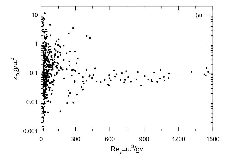
The roughness length with respect to the wind velocity made dimensionless with the Charnock length scale,  $z_{0u}g/u_*^2$ , versus the surface Reynolds number,  $Re_s = u_*^3/g\nu$ . Symbols show data from measurements taken over Kossenblatter See, Land Brandenburg, Germany, 6, 13 and 15 August and 12 October 1999. Horizontal line shows the Charnock formula with  $C_{ch} = 0.1$ .
