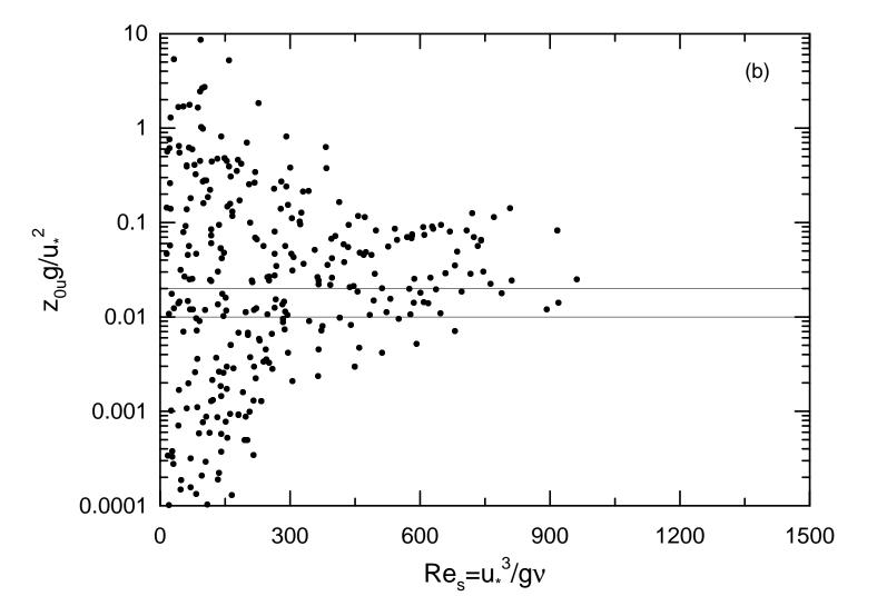
The roughness length with respect to the wind velocity made dimensionless with the Charnock length scale,  $z_{0u}g/u_*^2$ , versus the surface Reynolds number,  $Re_s = u_*^3/g\nu$ . Symbols show data from measurements taken over Baltic Sea, Field Station Östergarnsholm, from 1 November to 30 November 1998. Horizontal lines show the Charnock formula with  $C_{ch} = 0.01$ and  $C_{ch} = 0.02$ .
