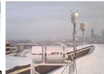
MTP-5 temperature profiler and its principle of operation
