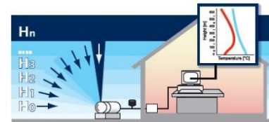
MTP-5 temperature profiler and its principle of operation
