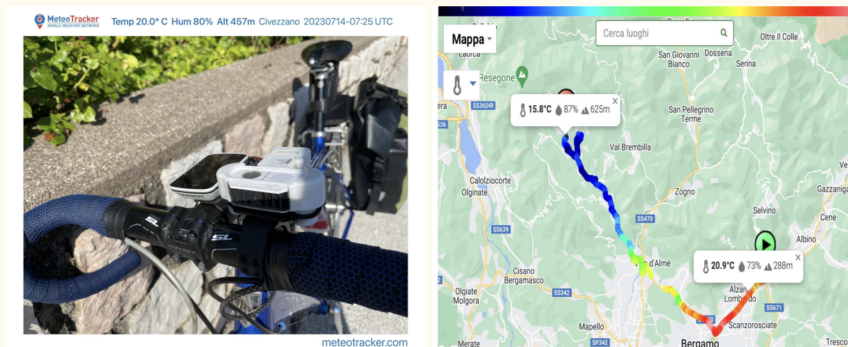
Figure 2. Analysis of the mobile PWS sensor Meteo Tracker showing the sensor attached to a bicycle (left) and a map showing the meteorological data gathered along the route taken (right), (images courtesy of Francesco Sudati).
