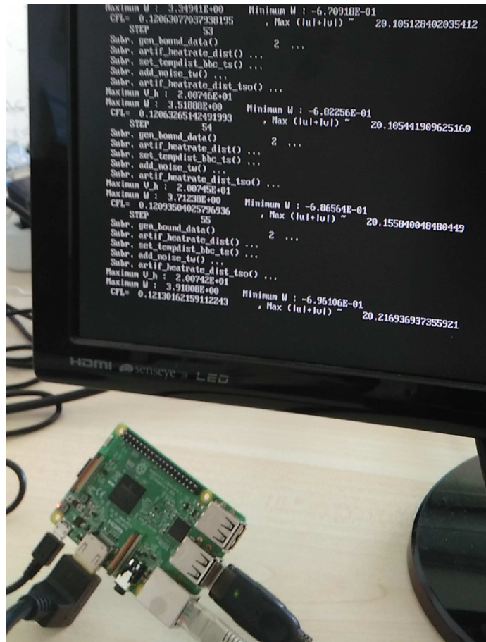
Figure 1: The Raspberry Pi connected to a huge screen, caught while running the COSMO model.
