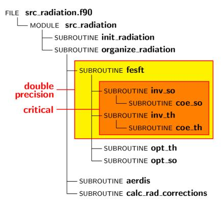
FIGURE 4: Structure of the source file *src\_radiation.f90*. The subroutines are nested according to how they call each other, the called subroutines indented with respect to the caller. The orange box encloses the subroutines that are critical with respect to precision, i.e. need to be run in DP regardless of the WP. The DP part has been expanded to what is enclosed by the yellow box due to performance considerations.
