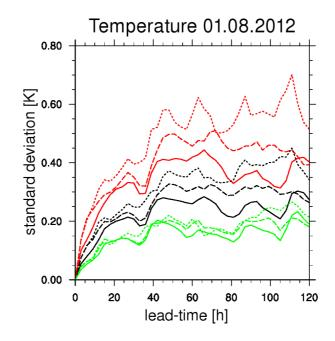
Figure 4: Ensemble spread for temperature averaged over the COSMO-E domain, at 500 hPa (solid line), 700 hPa (dashed line), 850 hPa (dotted line) and for experiment large (red), medium (black), small (green). Forecast initial date is 01.08.2012 00 UTC.
