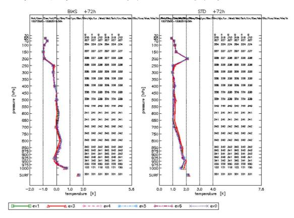
Figure 7: Bias (left) and the square of standard deviation error (right) of the upper air verification of temperature for one month in summer, using all stations in the COSMO-E domain.
