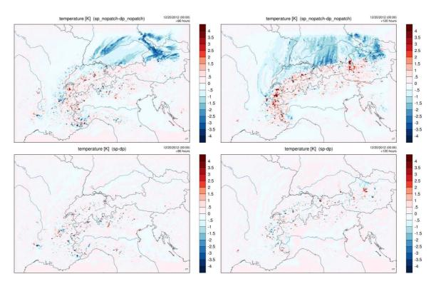
FIGURE 11: Difference in temperature between SP and DP with (top) and without (bottom) the winter bug after 96h (left) and 120h (right). (Top) The anomalies start to grow in specific places such as NW of Switzerland roughly parallel to the Jura mountains and along the Danube river valley, and from there grow by NE-ward advections. (Bottom) With the winter bug patch, the large deviations have disappeared, and only small, noisy signals over the alpine region remain.
