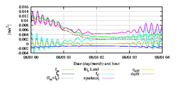
Figure 1: Terms of TKE equation in a stable case in the proximity of  $Ri_f = Ri_c$ .  $Ri_c$  is exceeded at around 01:00 when " $Ri_c$  Lim" line is above the " $f_m + f_h$ " line
