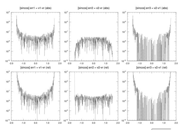
FIGURE 2: Numerical error in SP compared to  $\cos_x = \cos(x)$  in DP of  $\cos_x = \sqrt{1 - \sin(x)^2}$  (left) and  $\cos_x = \cos(x)$  (center), as well as the difference between them (right). The difference corresponds to the gain in precision when substituting  $\cos_x = \sqrt{1 - \sin(x)^2}$  by  $\cos_x = \cos(x)$ . The top panels show the absolute error, the bottom panels the relative error.
