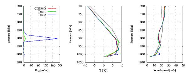
Figure 5: Vertical profiles of momentum diffusion coefficient(left), temperature (centre), and wind speed (right) at SPC site, on the 08/01/2012 at 00:00. Grey line represents the radiosounding observations, if present. Red line is COSMO default, green line is COSMO with  $K_{M,H} = 0.01m^2/s$  (Test 1) and blue line is COSMO with  $K_{M,H} = 0.01m^2/s$  and patlen = 0 (Test 2)
