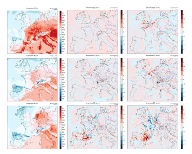
FIGURE 7: Results of the SP sensitivity experiments. Shown is temperature on the lowermost model level. Shown are the absolute field of OR (left), the deviations DP-OR (center), SP-OR (right). The lead times are 12h (top), 24h (middle), and 72h (bottom). The error growth is faster in SP than in DP with respect to OR, but the difference between DP-OR and SP-OR is already much smaller after 24h, and is gone after 72h, when they are of comparable magnitude.
