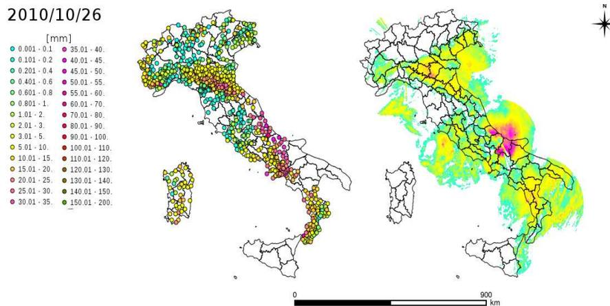
Figure 2: Rain gauges measurement (left) and pluviometric data from the Italian radar mosaic (mm/24h, 26th of October)
