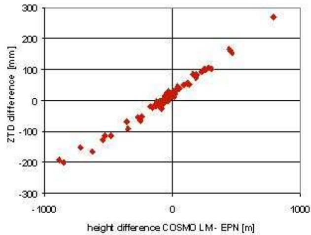
Figure 3: ZTD differences [mm] for EPN stations inside COSMO model in relation to height difference: EPN height (logs) - height of model ground level for station coordinates
