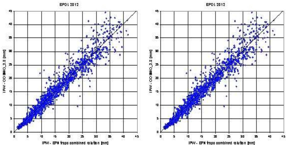
Figure 11: IPW comparisons GNSS EUR combined tropospheric solution for 2 GNSS stations in Poland vs. COSMO\_2.8 model (version I) in 2012 BPDL (Bielsk Podlaski) and LAMA (Lamkówko, near Olsztyn); correlations are respectively: 0.966 and 0.973 but difference standard deviation in each case around 2 mm
