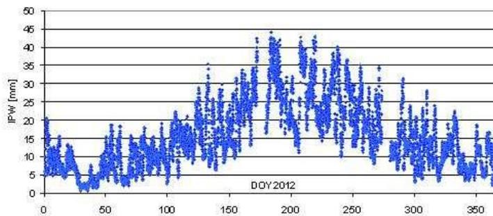
Figure 1: Precipitable water from EPN GNSS combined solution for station JOZE (Warsaw University of Technology Astro-Geodetic Observatory) in 2012
