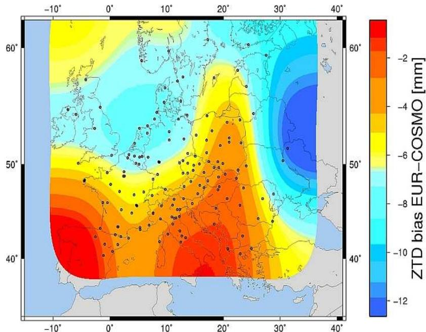
Figure 14: ZTD difference (GNSS EUR tropospheric combination - COSMO\_14; annual average) map for 2012, ZTD calculated by hydrostatical method
