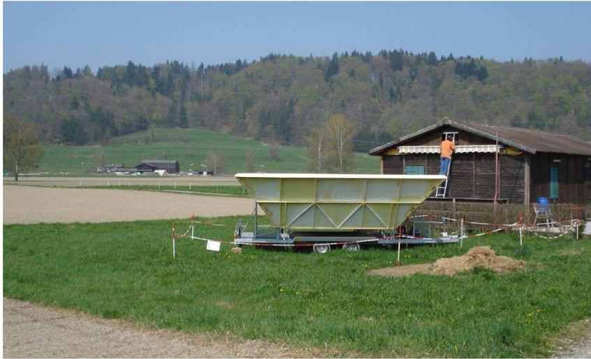
Figure 2: Vaisala mobile wind profiler during the second field campaign (March to June 2009) in the vicinity of the power plant of Mühleberg.
