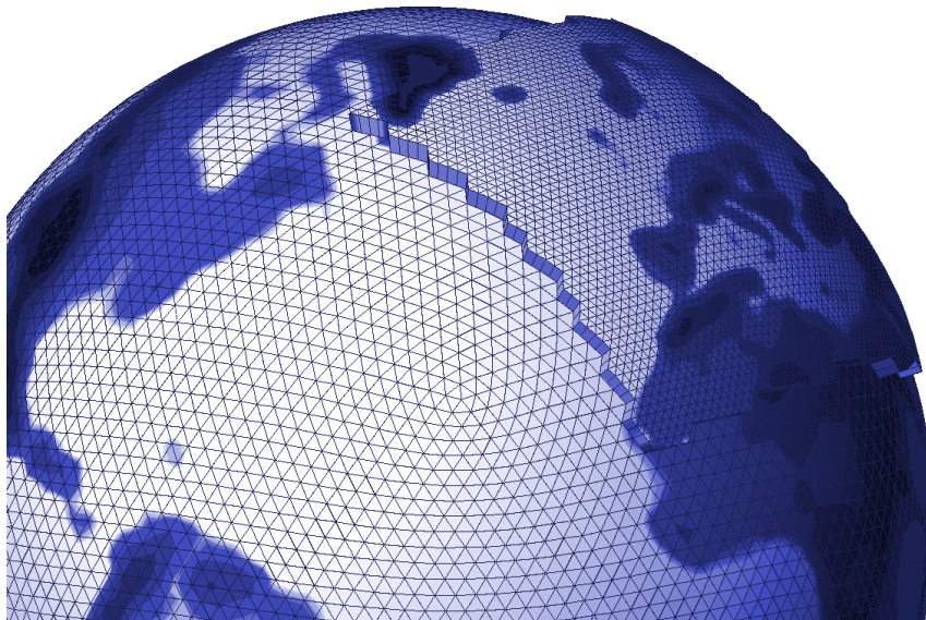
Figure 3.14.: Basic example of a multi-grid setup, consisting of a global ICON domain and a child domain over Europe with half grid spacing. This is similar to the deterministic forecast setup that is operationally used at DWD with a horizontal grid spacing of 13 km globally and 6.5 km in the child domain.
