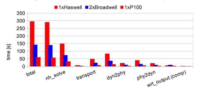
Single socket speedup, 1 Haswell CPU vs1 P100 GPU: 4.9x Source :W. Sawyer CSCS
