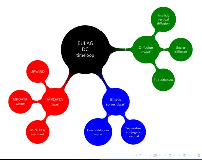
Implicit elliptic(Helmholtz) solver was optimized with the advent of the COSMO-EULAG compressible. MPDATA advection has been optimized within the ESCAPE H2020 project. The optimization of EULAG 3D diffusion has begun within the CEL-ACCEL project with the implementation of the 3D scalar EULAG diffusion operator for general grids.
