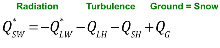
SW = short-wave LW = long-wave LH = latent heat SH = sensible heat
