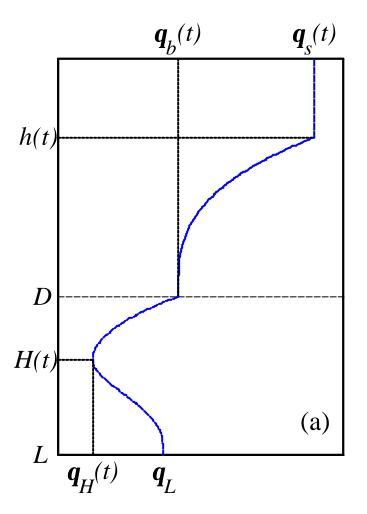
(a) The evolving temperature profile is characterised by five time-dependent parameters, namely, the temperature  $?_s(t)$  and the depth h(t) of the mixed layer, the bottom temperature  $?_b(t)$ , the depth H(t) within bottom sediments penetrated by the thermal wave and the temperature  $?_H(t)$  at that depth.
