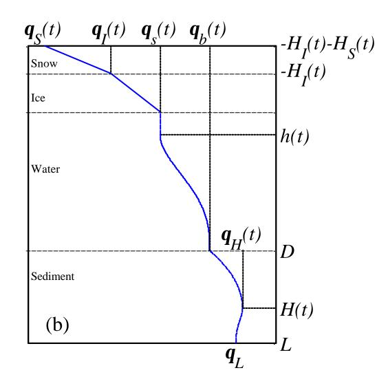
(b) In winter, four more variables are computed, namely, the temperature  $?_{S}(t)$  at the air-snow interface, the temperature  $?_{I}(t)$  at the snow-ice interface, the snow thickness  $H_{S}(t)$  and the ice thickness  $H_{I}(t)$ .
