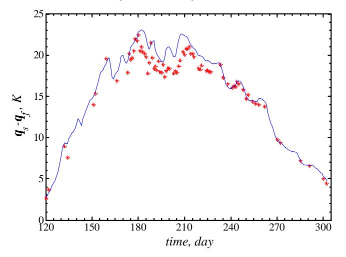
Water surface temperature  $?_s(?_f \text{ is the fresh-water freezing point})$ Dots – measured, Line - computed
